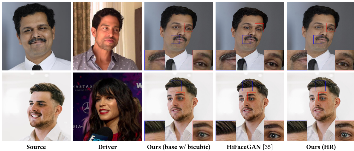
Figure 5: A qualitative comparison of different super-resolution methods applied to the output of our base model. While performing better than a baseline bicubic upsampling, we can see that the state-of-the-art super-resolution method (HiFaceGAN) cannot achieve the same level of high-frequency details fidelity as our approach. Digital zoom-in is recommended.
